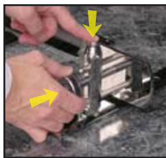
Depress the top button and push the knob until the Bier Pin plate is close to the casket or Commemorative Carriage.
